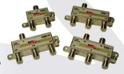
The SGHMQ Series Splitter is the ideal splitter for your Digital two-way plans. Designed to perform in systems utilizing Digital IP integration, cable modem and analog services where the highest isolation and RF performance are required. The Hi-Q design features SMT technology combined with high quality ferrites and blocking capacitors on all ports in for long term stability in performance. Available in 2, 3, 3B, 4 & 4T way configurations.
